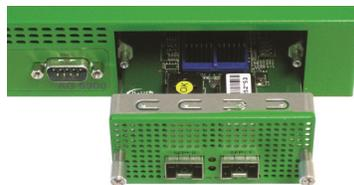
Figure 4 Inserting module
