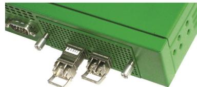
Figure 7 Removing transceivers
