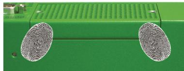
Figure 2 Blank filler plate removal
