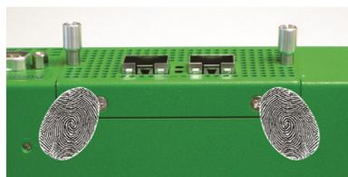
Figure 8 Removing module
