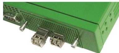
Figure 6 Inserting transceivers
