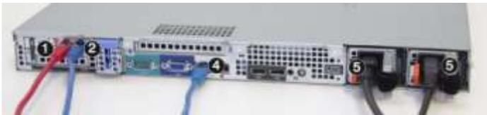
1. With the appliance powered off, install a crossover cable (red) between Alloc8's WAN port and the Router/Firewall.
